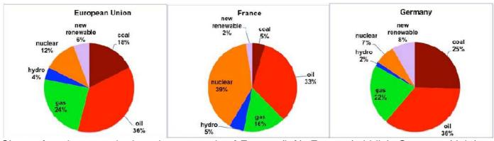
Share of each energy in the primary supply of Europe (left), France (middle), Germany (right) in 2012. Wind, photovoltaic, geothermal, biogas, and all renewables except wood, biofuels and hydro are in "new renewables". Wood is not included (7% of the supply in France).
