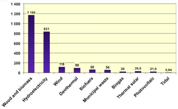
Renewable energy supply in the world in 2012, in million tons oil equivalent (with this unit the world consumption is around 13,000). Wood therefore represents 8% of the world total, and hydroelectricity 6% (primary energy equivalent).
